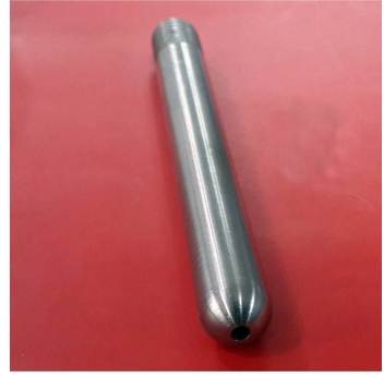
图 3 钢制简易模型照片,头部安装孔用于安装 PCB 传感器 Fig. 3 Steel simple model, the hole at the head is used to install PCB sensor
