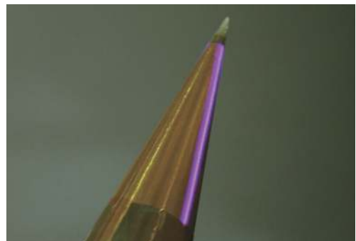
Fig. 12 The slender body model mounted in the wind tunnel and the discharge pattern of wire-based DBD plasma actuators
