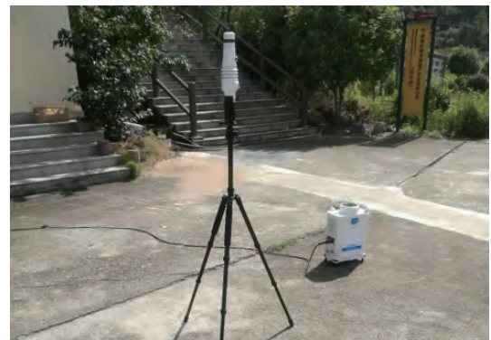
图 6 现场测量照片(左为手持气象站,右为激光测风雷达) Fig. 6 A photo of field measurements (the hand-held weather station and laser wind radar are respectively on the left and right)
